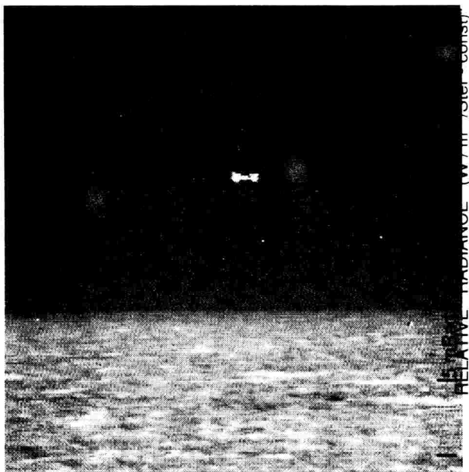
Fig. 1: NCCOSC aircraft (a) and row-averaged vertical radiance profile (b). The time is 4:42 pm with the sun low and far to the right and ASTD \approx -2.6^\circ C but Gulf Stream passing the tower. Water speckle is due to wave-slope-induced variability in reflected sky radiation and water emissivity. The radiance rise at the horizon is smoothed by atmospheric attenuation and path emission and is positive because the air is cooler than the water. [Scene ThAC2]
